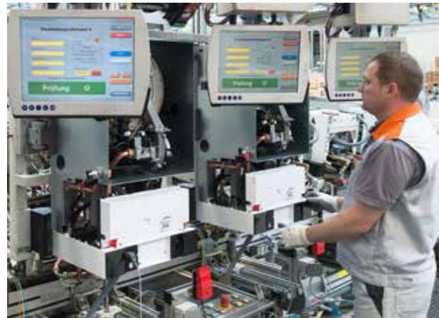
A test stand on a production line for wall-mounted gas boilers at corporate headquarters in Allendorf (Eder)
